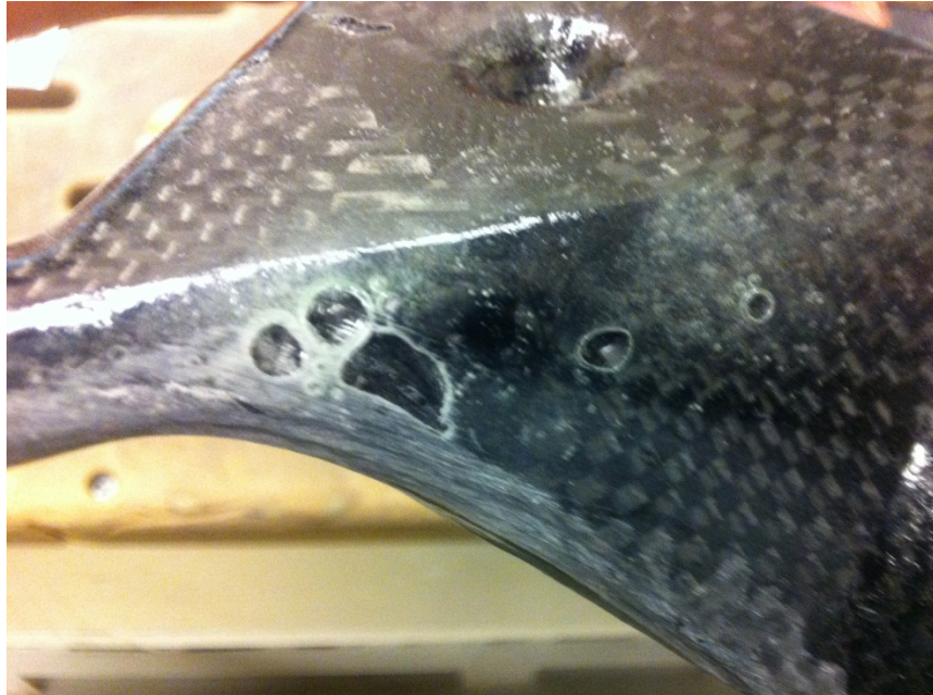
Figure 57 – Propeller parting line and voids in the epoxy
