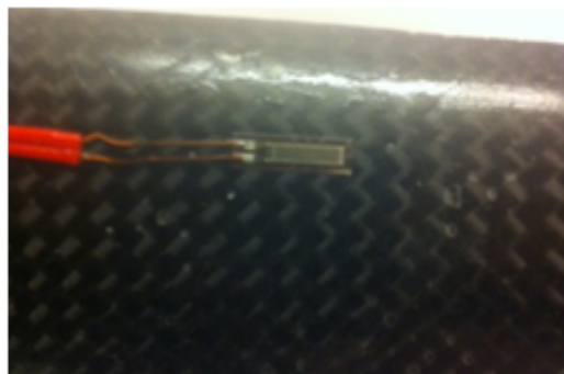
Figure 33 – Strain gage attached to the blade surface
