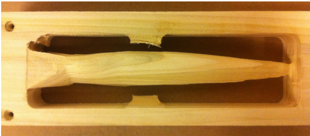
Figure 62 – CNC machining of wooden propeller blades
