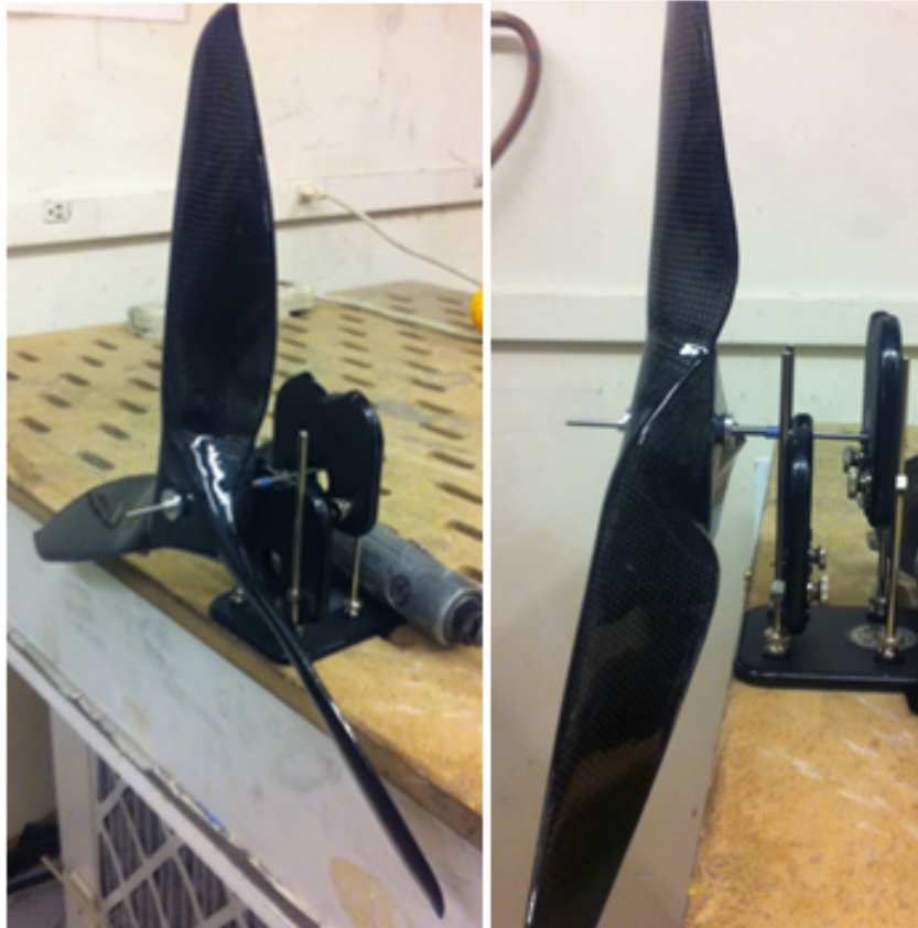
Figure 58 – Balancing 3-blade propeller
