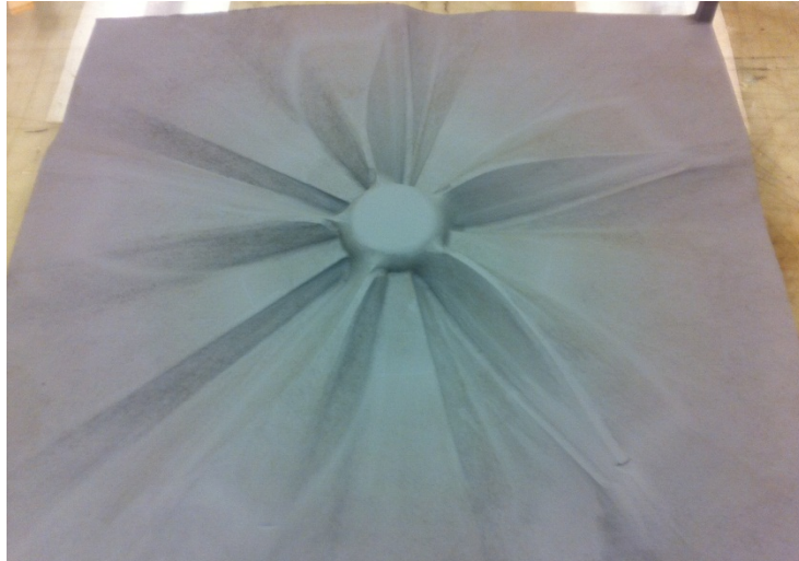
Figure 52 – Primer coating on 5-bladed propeller male mold plug
