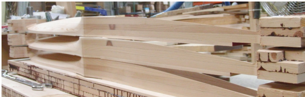
Figure 7 – Sensenich Wooden Propeller after front surface milled
