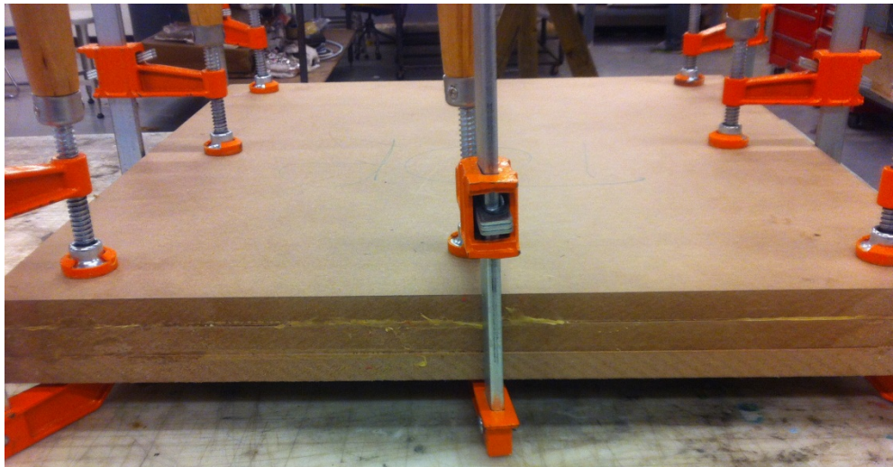
Figure 50 – Stacked and glued MDF board
