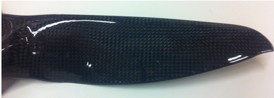
Figure 60 – Finished propeller blade after epoxy coating
