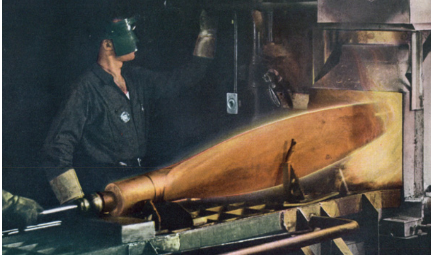
Figure 9 – Aeroprop worker heat treating steel blade (General Motors Corporation 1944:26)
