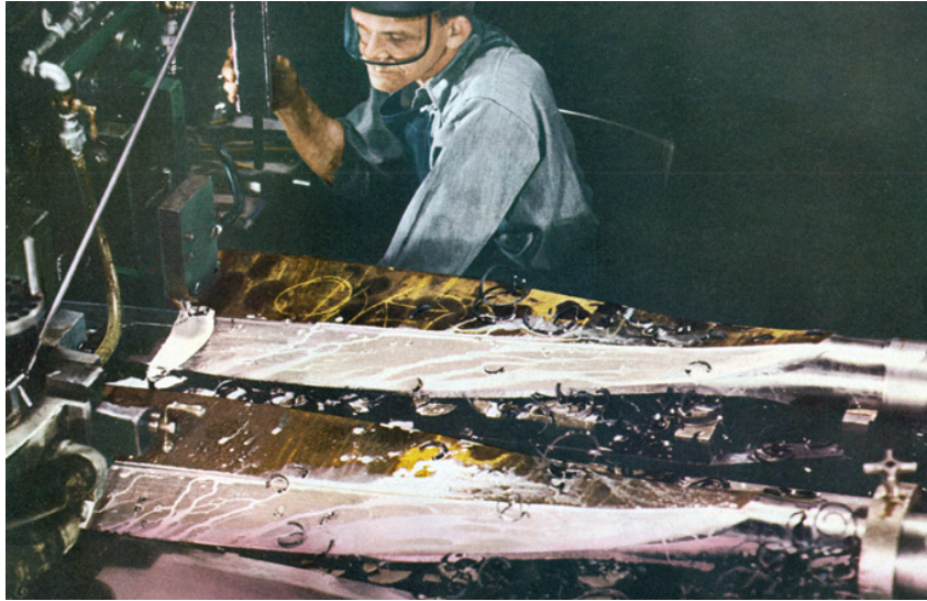
Figure 8 – Aeroquip worker using multiple planer on steel blade (General Motors Corporation 1944:25)
