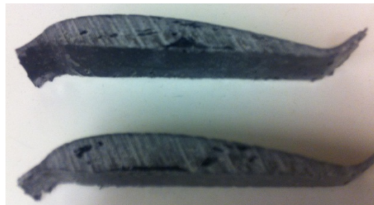
Figure 78 – Air pockets in chopped fiber core material
