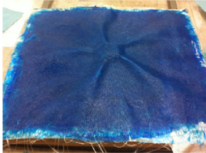
Figure 53 – Tooling fiberglass layers on 5-bladed propeller male mold plug
