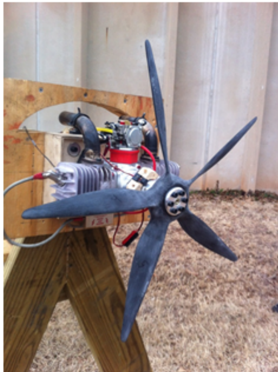
Figure 36 – DA-100 gas engine with 5-blade propeller
