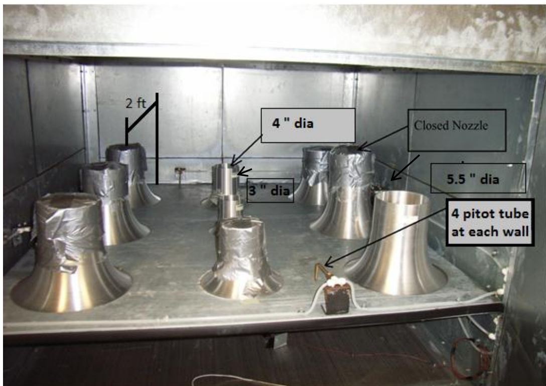
Figure 9: Nozzle bank inside code tester of indoor room
