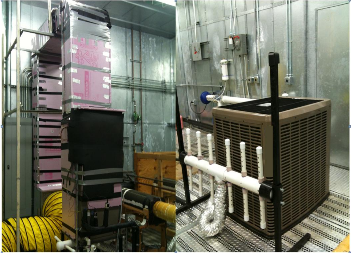
Figure 6: Indoor blower/coil assembly (left side) and outdoor condensing unit (right side)
