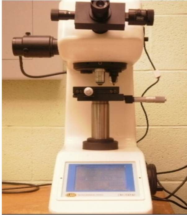
Fig. 2.7 Clark Microhardness tester.
