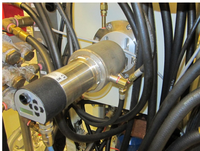
Fig. 2.5 Single color optical pyrometer to measure temperature of sample during SPS.
