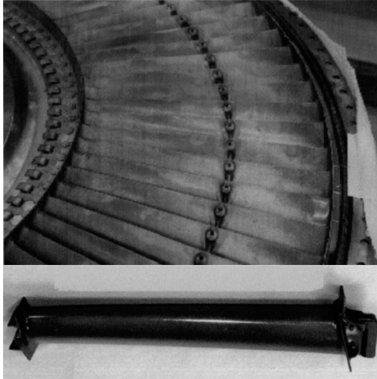
Fig. 1.8 Low pressure \gamma -titanium aluminides turbine rotor of CF6-80C engine (with permission from [37]).
