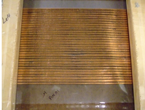
Figure 3.10b: Photograph of Comb Circuit
