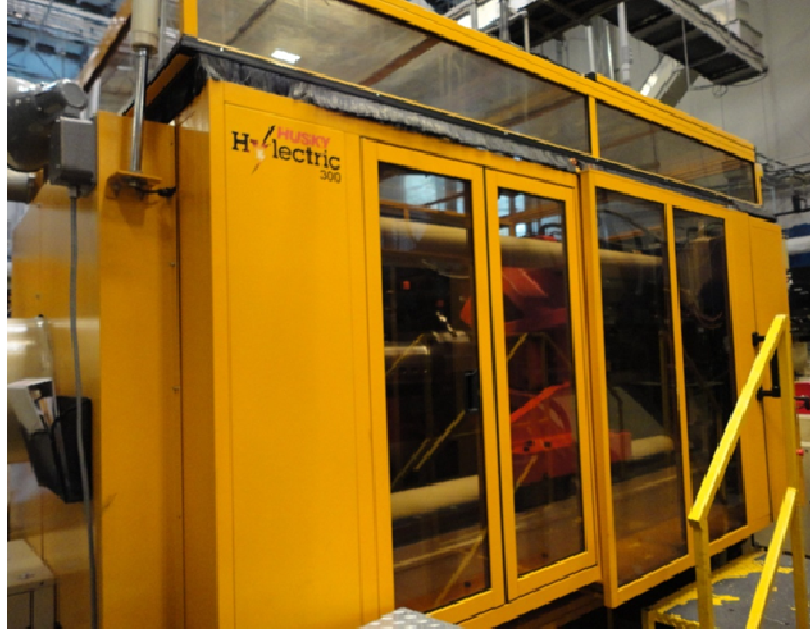
Figure 15: Caps were collected from Husky 300 Injection molding machine.
