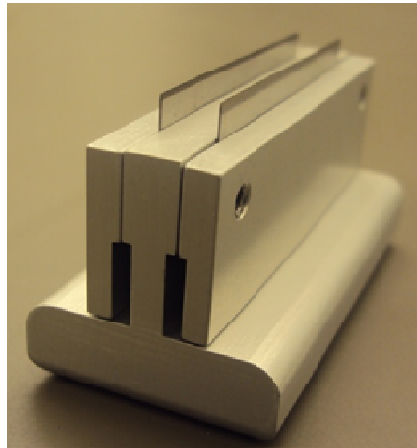
Figure 13: Parallel cutter used to ensure uniform width of the samples.
