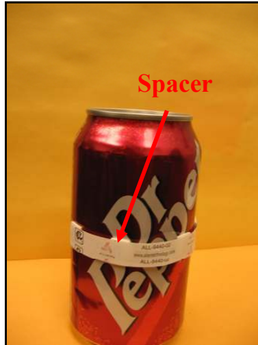
Figure 45: RFID tag slapped on metal can using spacers
