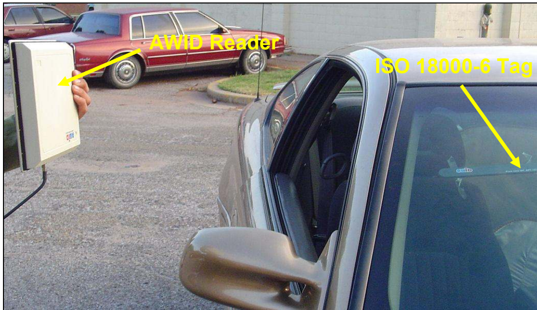
Figure 11: Tag-Antenna (AWID) Setup for Experimentation
