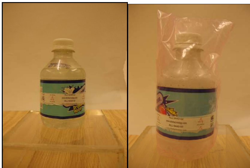
Figure 25: Placement of tag on plastic bottle containing organic liquid (water) and plastic bottle stored in plastic bag
