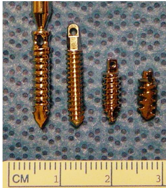
Fig 1. Photograph of the suture anchors tested from left to right: Securos 3.5mm, FlexiTwist 3.5mm, IMEX 4.0mm, Fastin 4.0mm.
