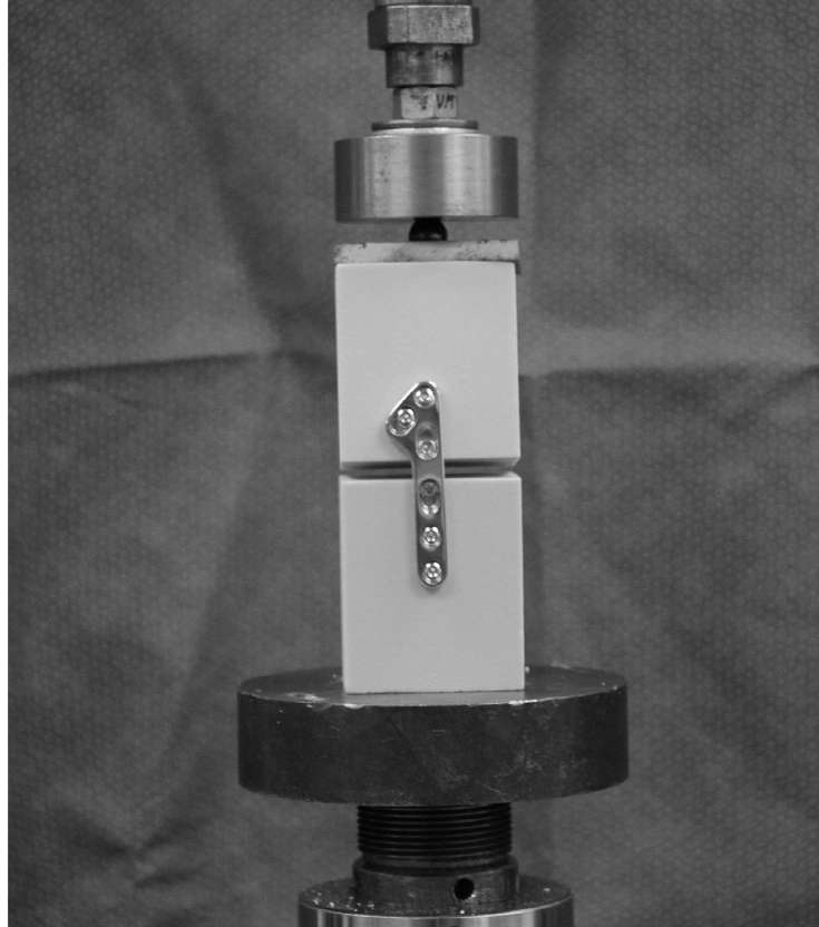
Figure 1: View of a LocP construct positioned and loaded in the material testing system prior to axial compressive load to failure testing. Note the customized loading platform atop the construct.
