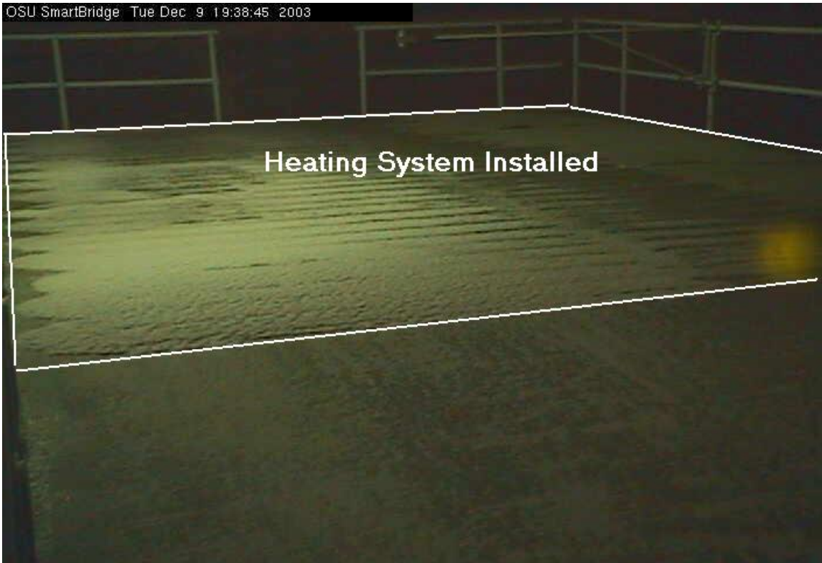
Figure 4-6: Event 1 Bridge Snapshot at 19:38, 12/9/2003 (Snow, +3 hours)
