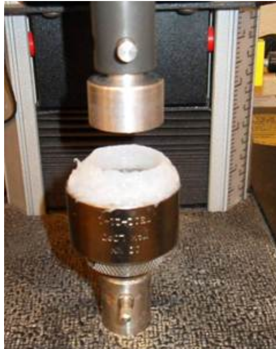
Figure 3.2. Custom made top and bottom compression testing anvils with hydrogel chamber used on the INSTRON 5542 machine.
