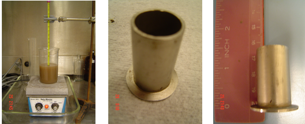
Fig 7.2: (a) Fouling experimental set up (b) Stainless steel tube insert (c) Top view of inset
