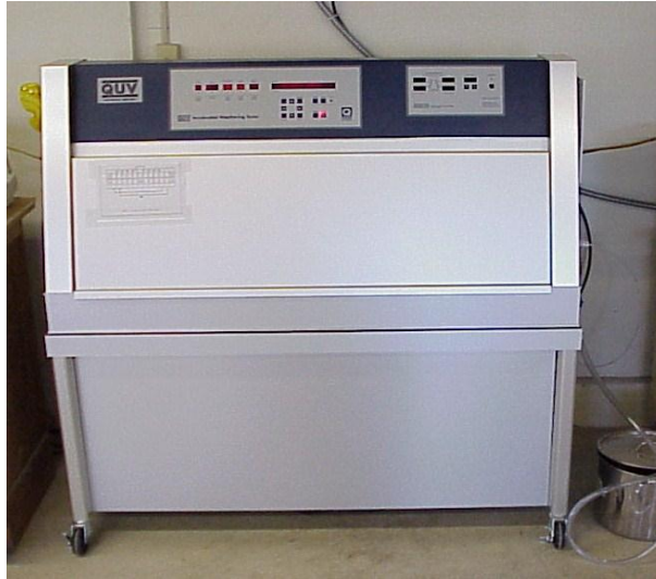
Fig. 4.15 An image of the weatherometer (artificial weathering chamber) used.
