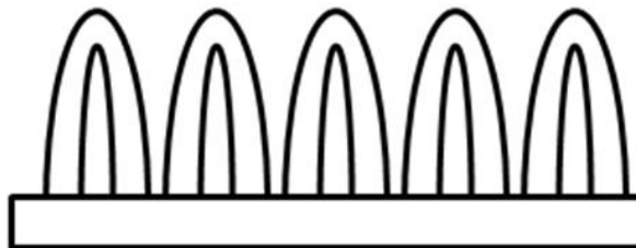
Fig 2.4 An illustrative diagram of loop - pile type carpet (when the loops are cut, you remain uncut) [16]
