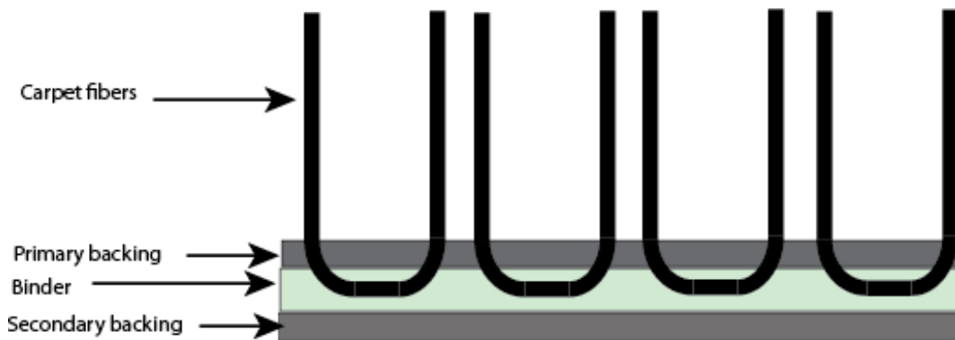
Fig. 2.1 An illustrative diagram of carpet (cut- pile type) and its constituents – fibers, backing and binder [4].
