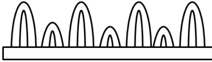
Fig. 2.5 An illustrative diagram of patterned loop type carpet (when the loops are uncut and have multiple heights) [16]
