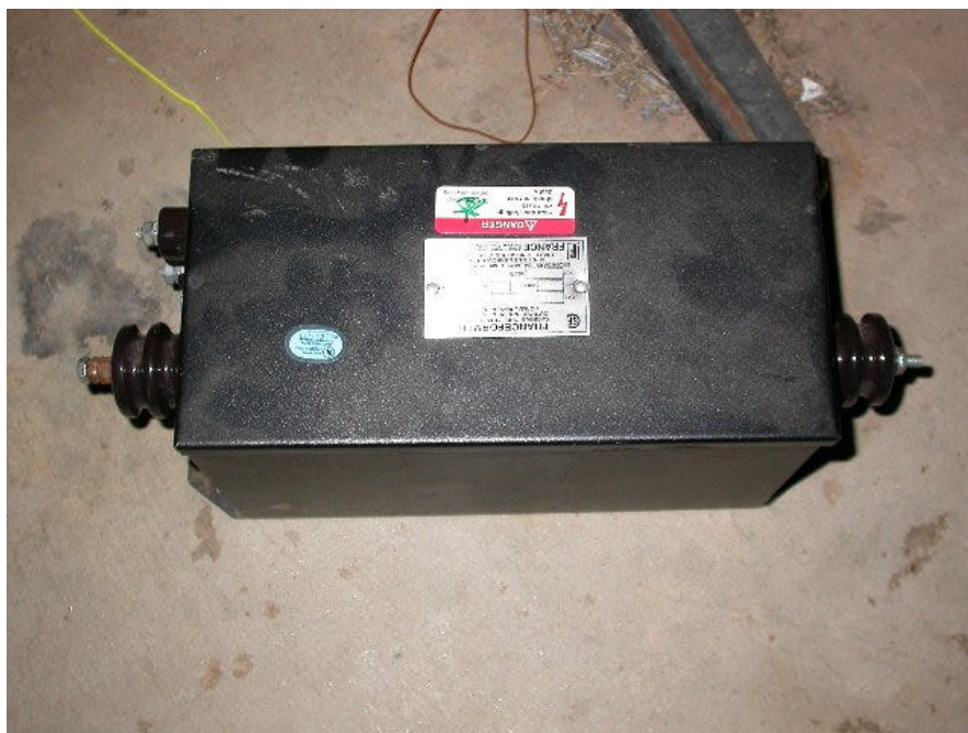
Figure 3.12. Franceformer Model 15060P Transformer.
