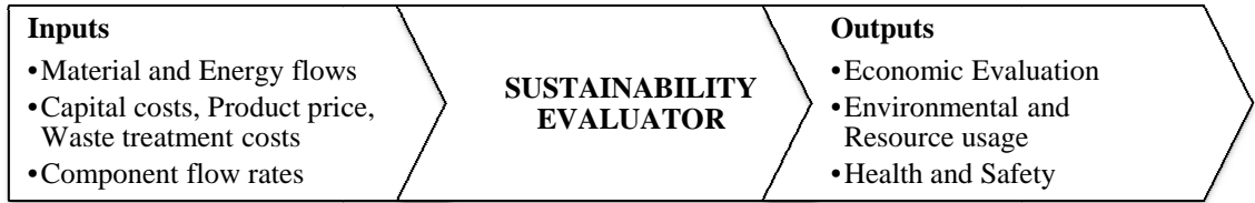
Figure 2.1 Functioning of the SE
