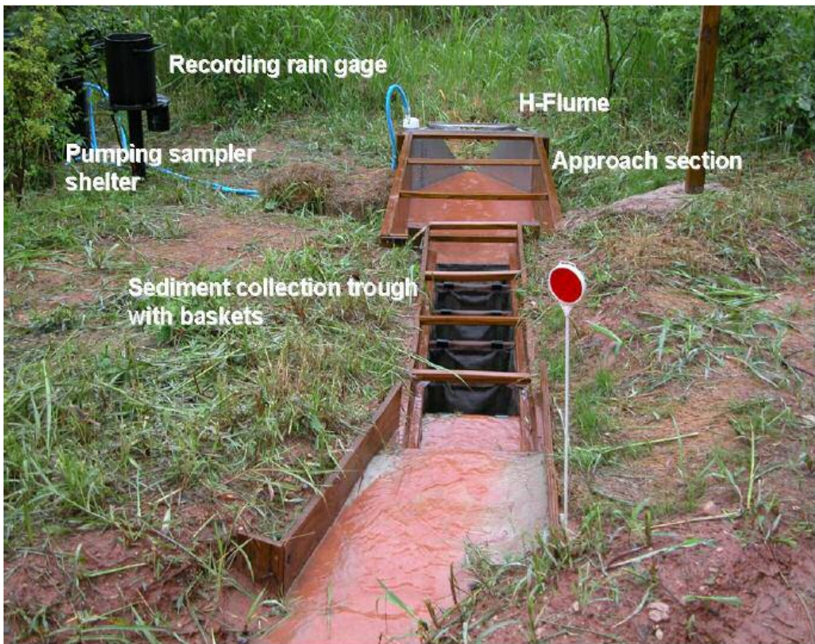
Figure 2. Components of the sediment collection stations used to measure erosion from each road segment.
