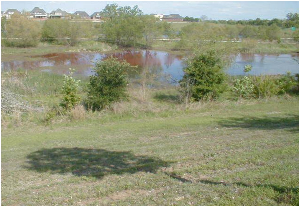
Figure 10: Dye observation during 4/25/05 event shows the heterogeneous nature of the dye dispersion in the wetland. The dye-tinged band of water in the background illustrates the preferential flow path.
