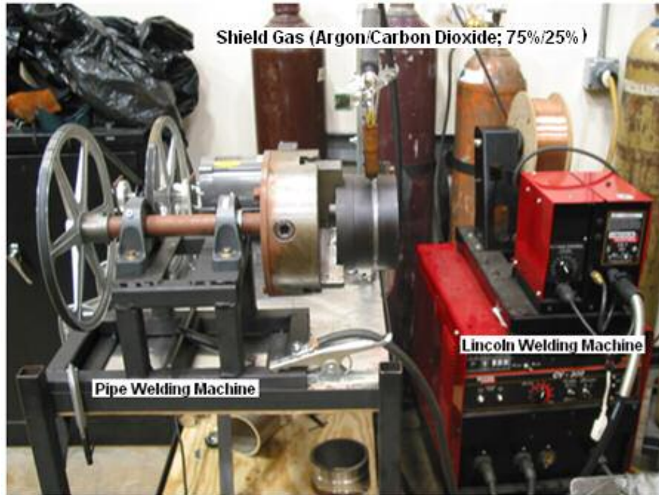
Figure 4.2: Complete pipe welding machine and Lincoln Electric welding machine setup
