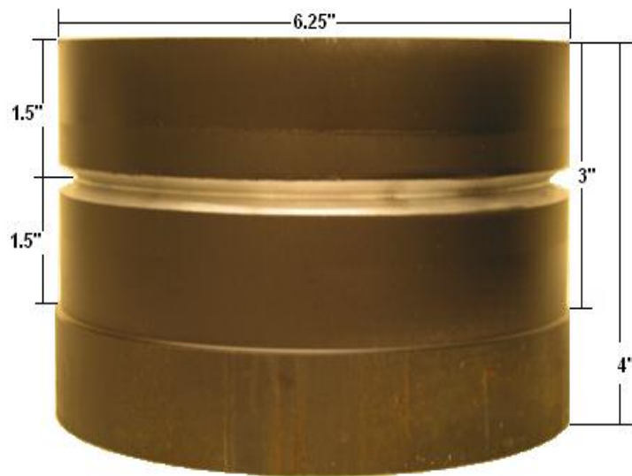
Figure 4.7: Machined and painted workpiece with a finished V-groove
