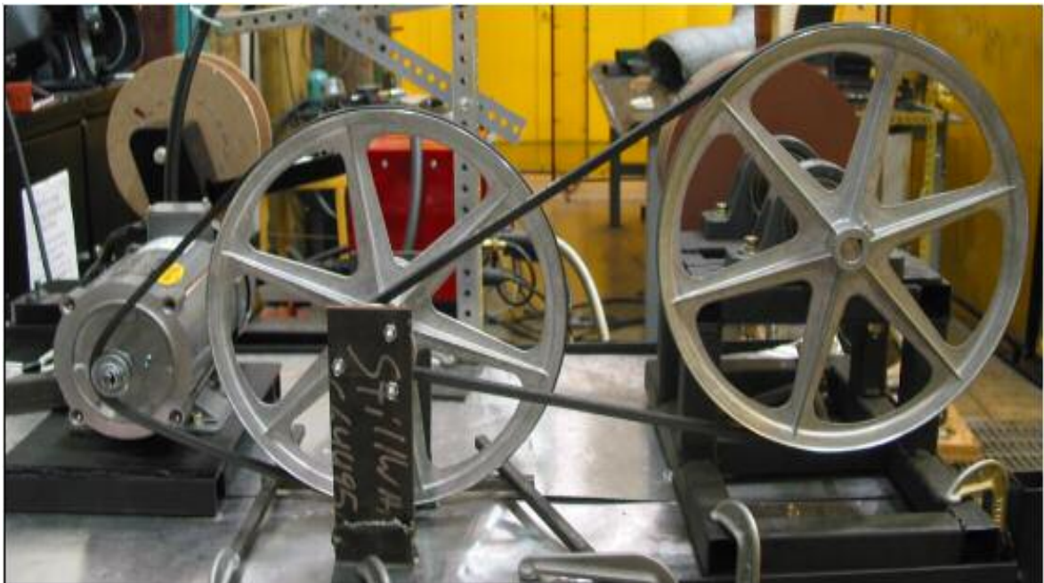
Figure 4.3: The motor as connected to the belt and pulley system on the pipe welding machine
