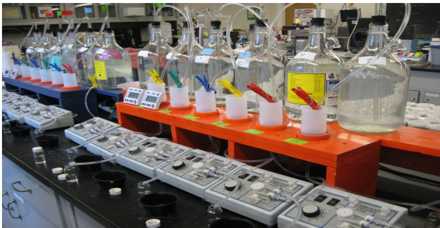
Fig. 1.3: Complete flow-through set-up with Mariotte bottle, flow-through column, and single channel pump.
