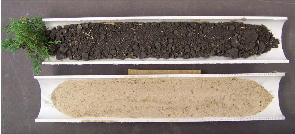
Figure 4. Two of four wind tunnel treatments for the Fall 2009 semester, bare sand and organic soil with a windbreak.
