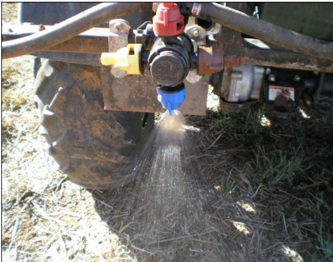
Appendix Figure 8. Flat fan nozzle for the topdress application of liquid UAN.
