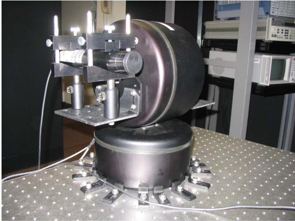
**Figure 4.3 Helium-neon laser mounted on Model-20 Pan and Tilt gimbal.**
