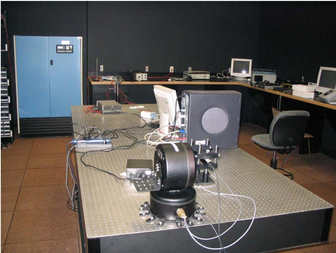
**Figure 4.2 Gimbal repeatability and accuracy experimental setup viewed from behind the gimbal towards the PSD.**
