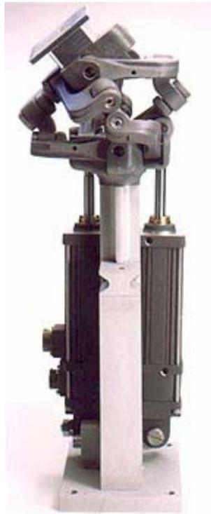
**Figure 2.9 Omni-Wrist III Sensor Mount [38].**
