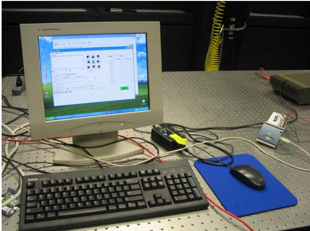
**Figure 4.4 Control computer and PMD-16008FS data acquisition device.**
