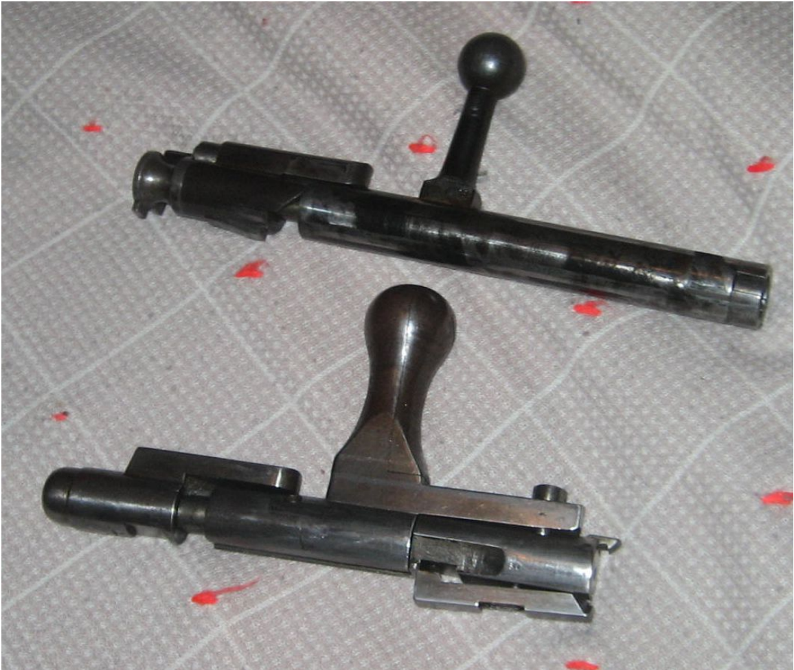
Figure 8: The Bolts From Dutch Model 1871/88 and German Model 1888 Rifles
