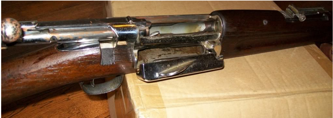
Figure 14: The Action of a United States .30-caliber Model 1898 Krag-Jorgensen
