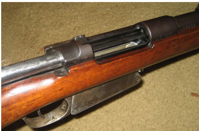
Figure 15: The Action of an Argentinean 7.65mm Mauser Modelo Argentino 1891 Close up of the action on a German-made export Argentinean Mauser, caliber 7.65mm, made in Berlin in 1899. This rifle and the proceeding Belgian 1889 and Turkish 1890, all three of similar design and caliber, were the first Mauser smokeless repeating rifles,
