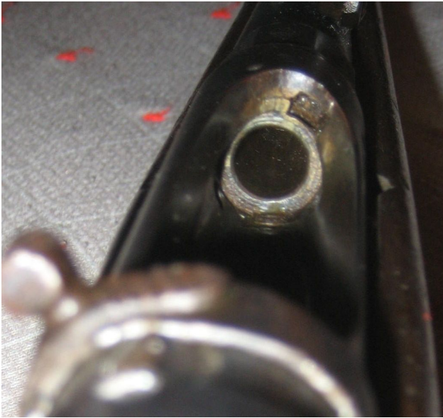
Figure 10: The Tubular Insert of the 6.5mm Fucile Mo. 1870/87/15 Vetterli-Vitali
