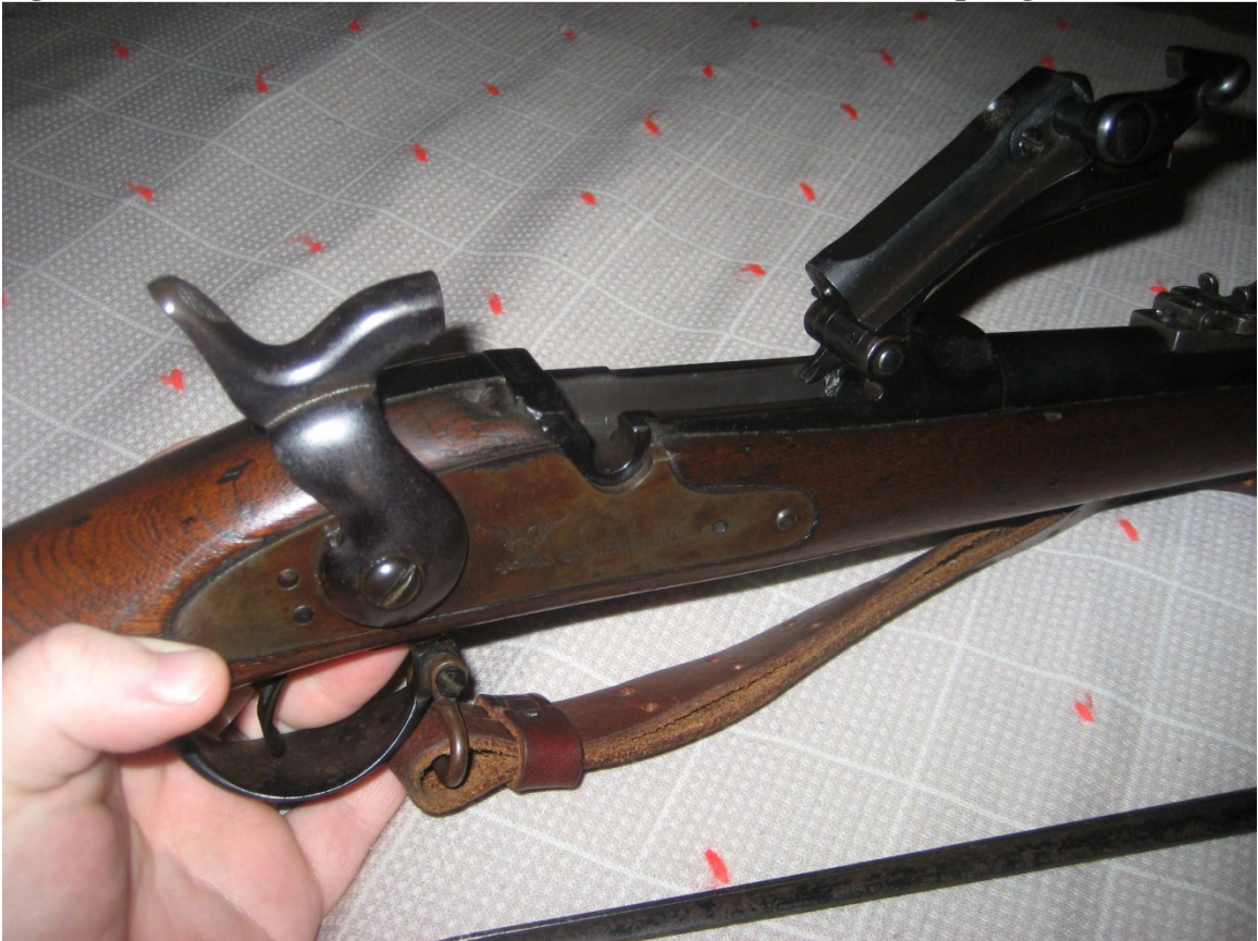
Figure 6: The Action of a United States .45-caliber Model 1873 Springfield Rifle
