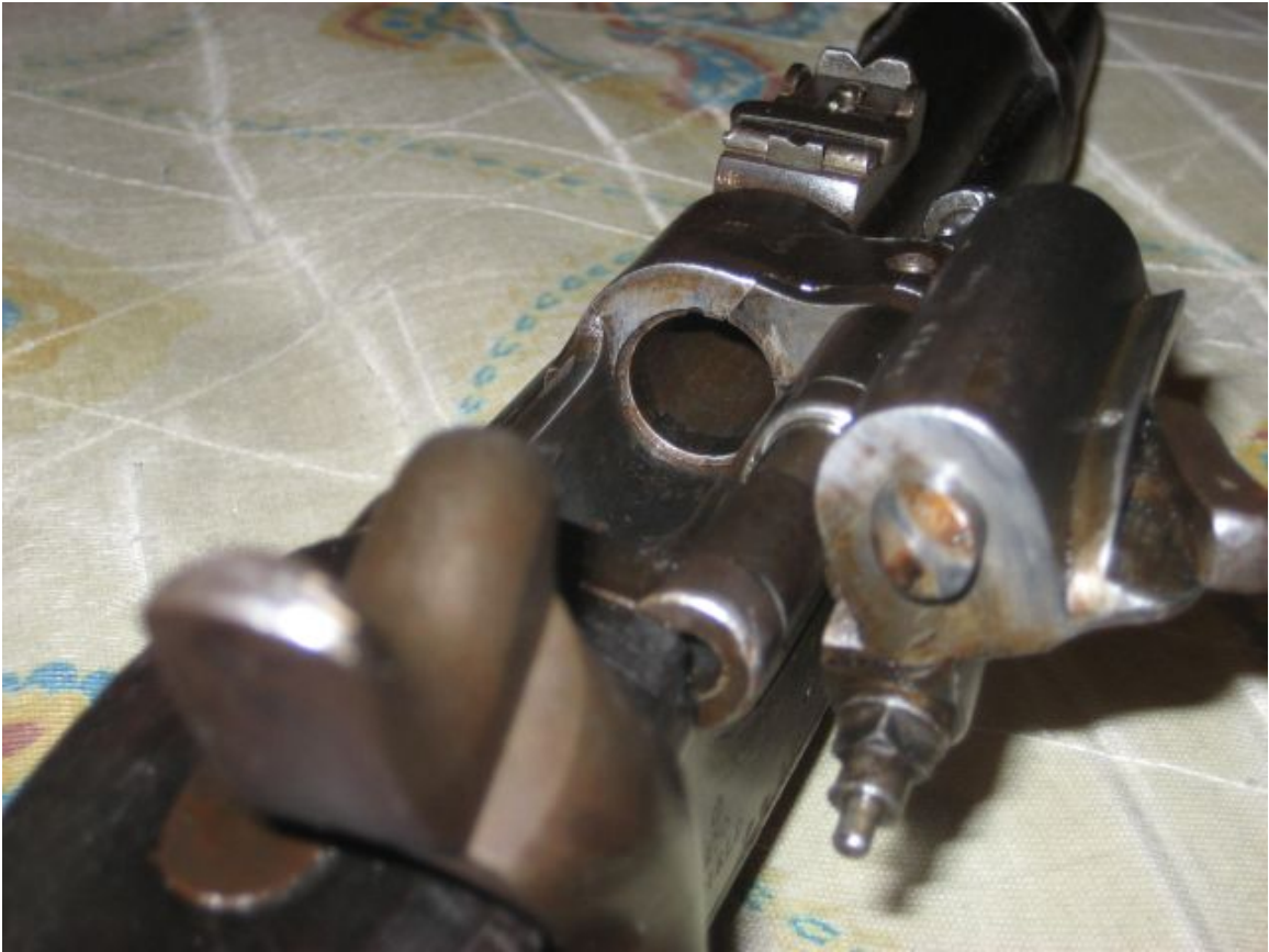
Figure 2: The Action of a British .577-caliber Snider-Enfield Mark III Carbine
