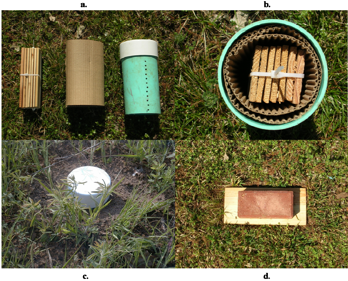
Figure 3.1. (a) In-ground monitoring station components including wood ‘sandwich’, cardboard, and PVC pipe, (b) assembled in-ground monitoring station (top view), (c) emplaced in-ground monitoring station, (d) emplaced soil-surface ground-board.
