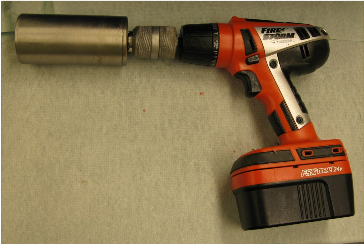
Figure 3. After exiting the Ross Integrated Tenderizer, beef cores were extracted using a 5.08 cm (20.25 cm 2 ) stainless steel circular drill bit from each subprimal.
