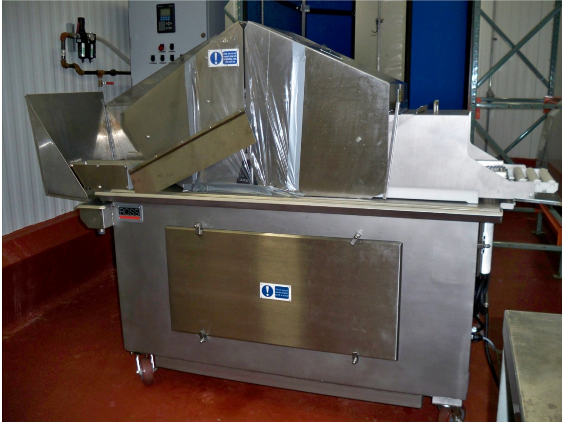
Figure 2. Ross tenderizer TC700MC equipped with a custom-built Dositron multi nozzle spray system .
