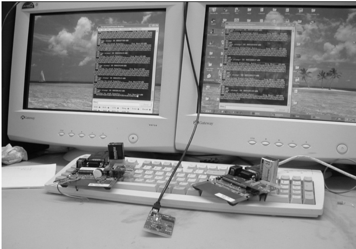
Figure 4-2 Experimental setup in the lab (Device on the left side is the End device with sensor, in the middle is a Packet sniffer, device on the right side is the Coordinator, which we use to collect data.)
