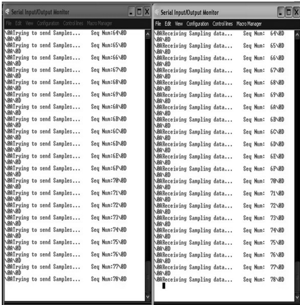
Figure 5-2 Traffic monitoring after modification (Left side window is monitoring the End device; right side window is monitoring the Coordinator side)
