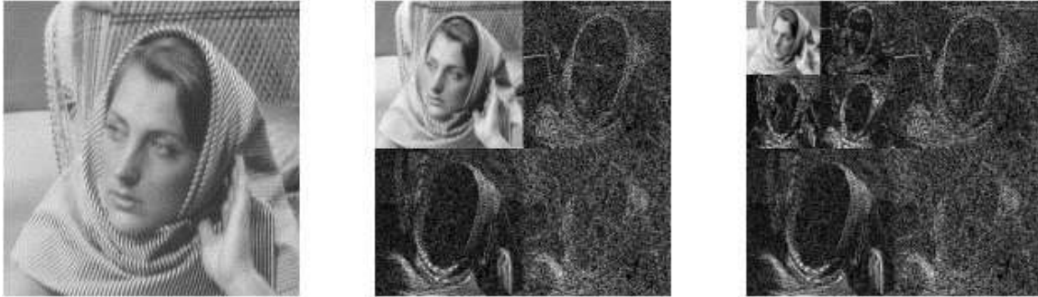
Figure 1. Wavelet compression example
