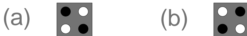
Figure 1: The darkened dots represent the location of the electron in a given cell. The two cell states are represented here, (a) shows polarity P=-1 (binary 0) and (b) with polarity P=+1 (binary 1)
