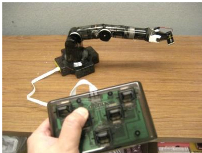
Figure 1: OWI007 Robotic Arm with remote control
