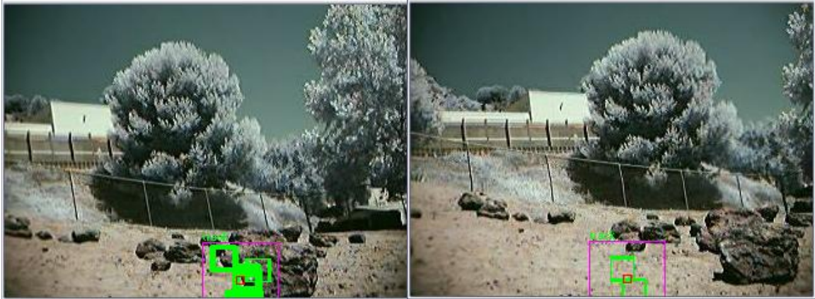
Figure 11: Example of tracking a single point on successive frames on a rock in the JPL Mars Yard. The target changes in the second image but the number of hits still remains high.
