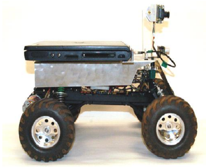
Figure 5: Assembled configuration with USB webcam and laptop computer [23].
