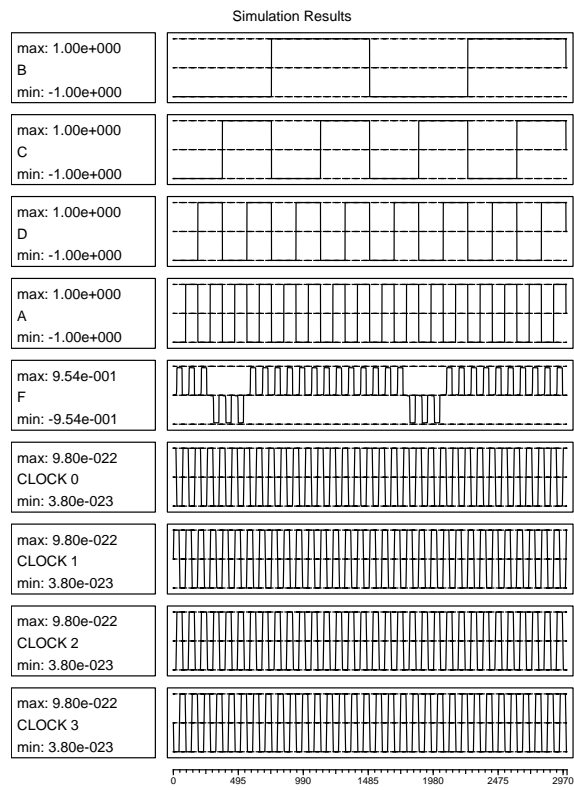
Figure 3.3: QCA-based TH34W2 gate and its waveform.
