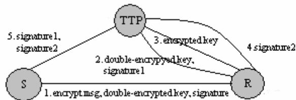
Figure 2.2: Secure message Transfer Protocol for E-commerce
