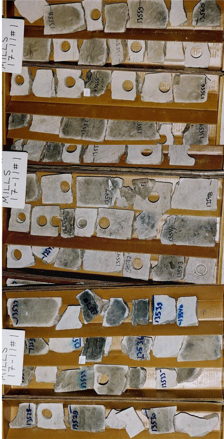
Photographs of core from the T.R. MILLER MILLS 17-11, #1 well of the Conecuh Embayment of depth between **13528-13560 ft** dominated by oolitic packstones and grainstones facies.
