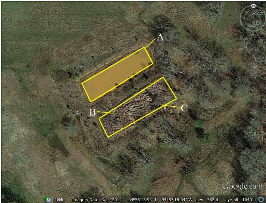
Figure 6 Aerial photo of the Le Bosquet passive treatment system (Google Earth 2013). Each letter represents a sample point for each outflow as follows A=ALD, B = Ox, C = VegWL.
