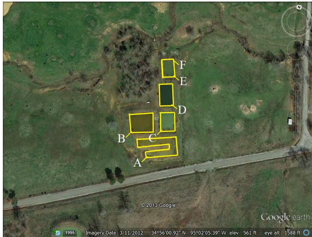
Figure 7 Aerial photo of the Red Oak passive treatment system (Google Earth 2013). Each letter represents a sample point for each outflow as follows A=ROW1, B = ROW2, C = ROW3, D = ROW4, E = ROW5, F = ROW6.
