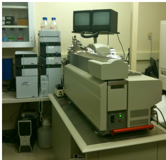
Figure 7. LC-MS/MS Used in Study Shimadzu HPLC system attached to an Applied Biosystems 4000 Q-Trap LC-MS/MS System in the Oklahoma State University laboratory.
