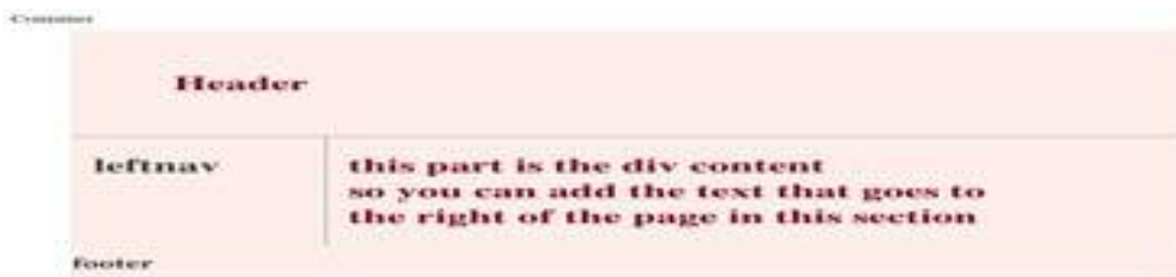
Figure 4.10. By applying a left margin to the right column, the content of the right column starts to move to the right. Two columns have been created: the left column with the word "leftnav" in it, and the right column with text in it
