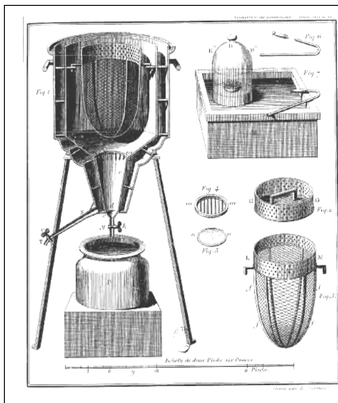
Fig. 7-5. Ice calorimeter designed by Laplace and Lavoisier to measure caloric and fixed air (carbon dioxide) during a chemical combustion or animal respiration. Left: the calorimeter contained three concentric chambers. In the inside chamber a burning object or a respiring animal was producing caloric, which could melt a specific quantity of ice held at the middle chamber. The outer chamber was filled with snow as an insulator. The quantity of the melted ice in the middle chamber was proportional to the heat produced in the inside chamber. From Lavoisier's Mémoires de chimie et de physique (Paris: 1862).
