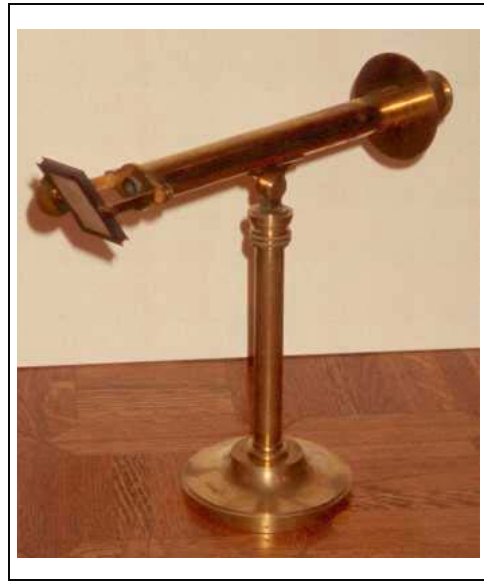
Fig. 7-1. The polarimeter which Arago used to demonstrate the laws of light polarized by reflection and refraction, now preserved at the Millington-Barnard Collection, the University of Mississippi, USA.
