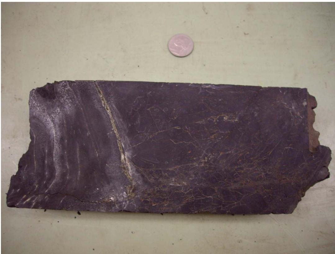
Figure 7. A section of the Black Shale subunit. Oxidizing pyrite cement in fractures give this sample the orange color. California Oil, Mullen et al #1. Depth 8,982 ft.
