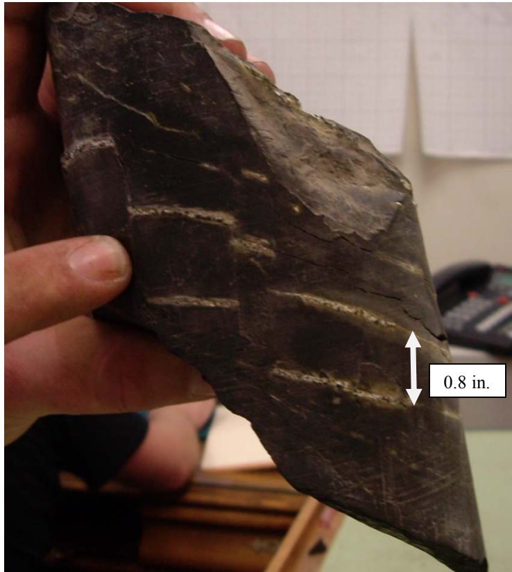
Image 100-586 Fractures cutting pyrite bands in the cherty subunit. Texaco, Drummond 1-K. Depth of 3047-3050 feet.
