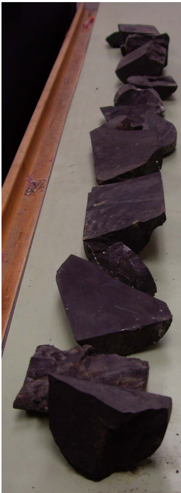
Image 100-571. Black shale subunit. Diameter 4.5 inch. California Oil, Mullen et al #1. Depth 9019-9023 ft.
