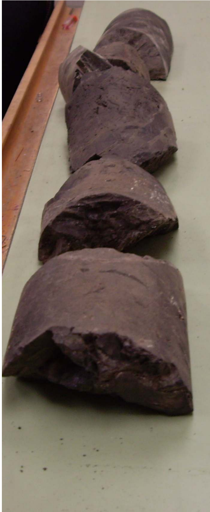
Image 100-572. Chert layering and color indicative of the Cherty subunit. Core diameter 4 inch. Texaco, Drummond 1-N, Depth 3052-55 ft.
