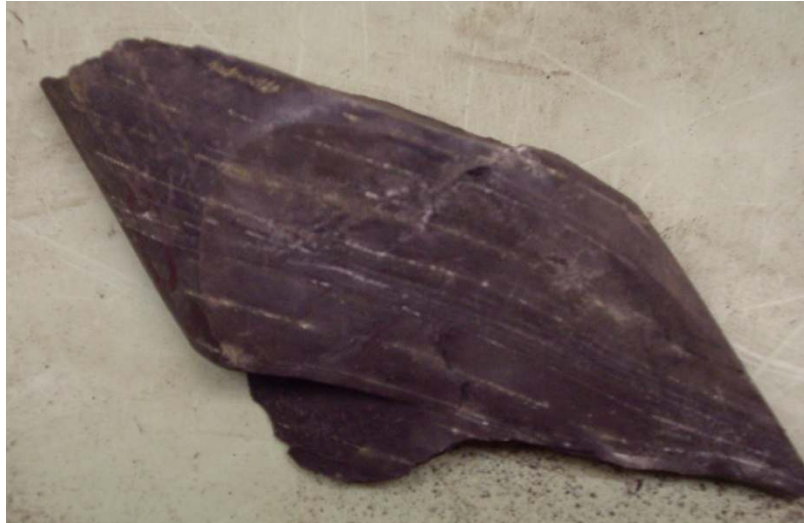
Image 100-596. Black shale subunit cemented with pyrite. California Oil, Mullen et al #1 from a depth of 8986 ft.
