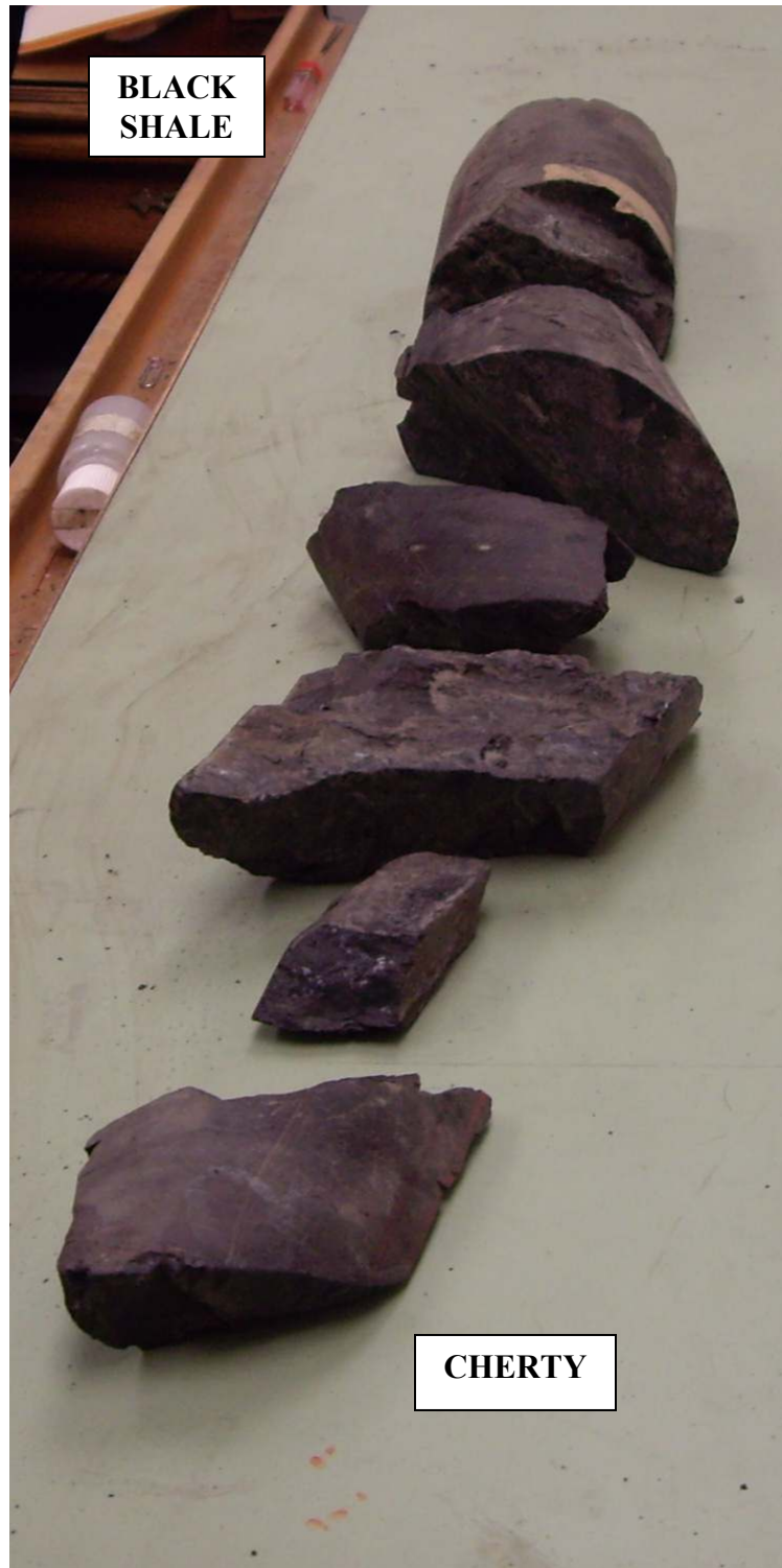
Figure 5. Contact of the cherty subunit (bottom of picture) and the black Shale unit (top of picture). Texaco Incorporated, Drummond 1-N. Depth 3067-2076 feet.
