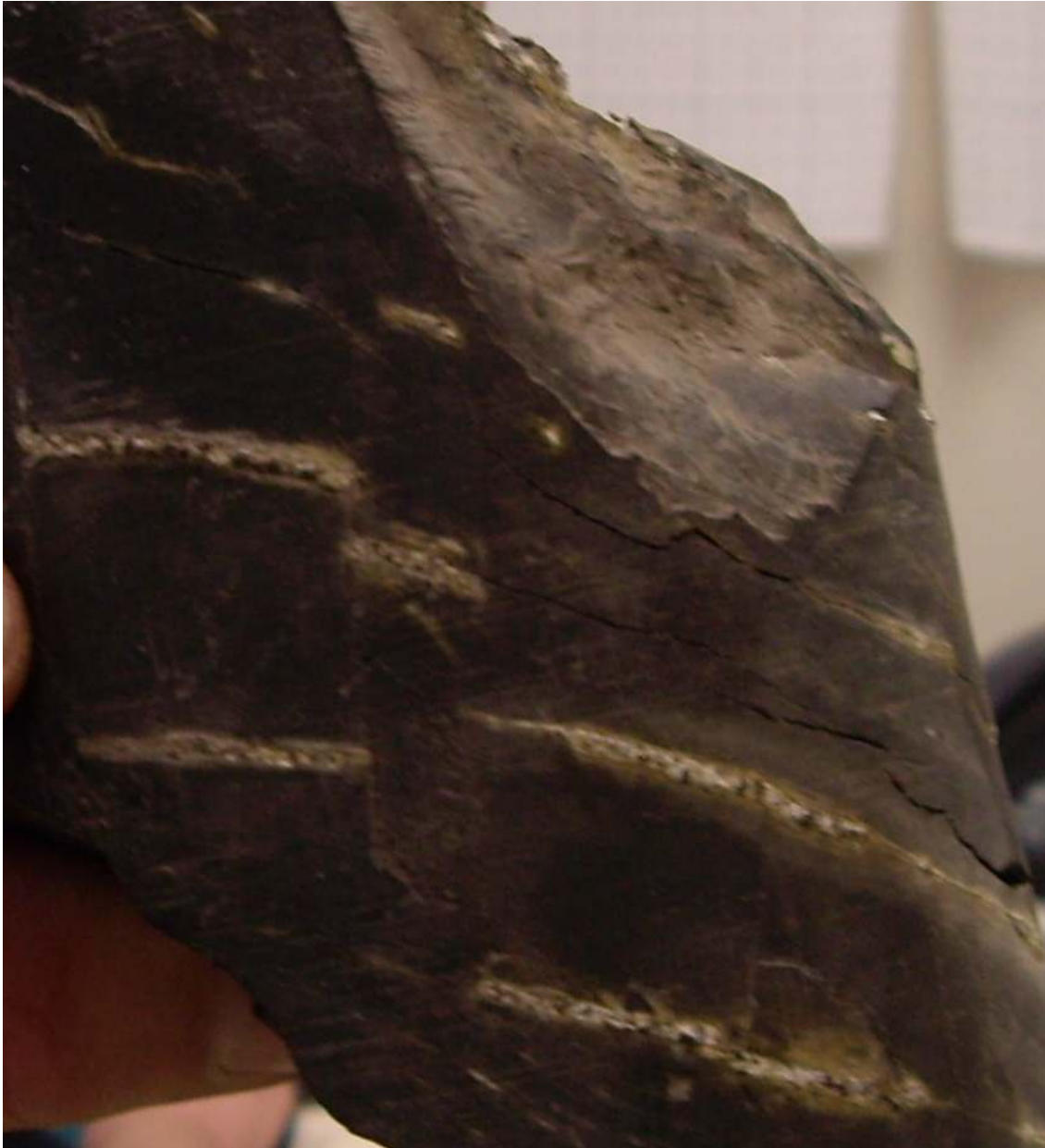
Figure 6. Fracturing of the Chert subunit. Micro-faulting offsets lighter colored pyrite bands. Texaco Incorporated, Drummond 1-K. Depth 3047-3050 feet.
