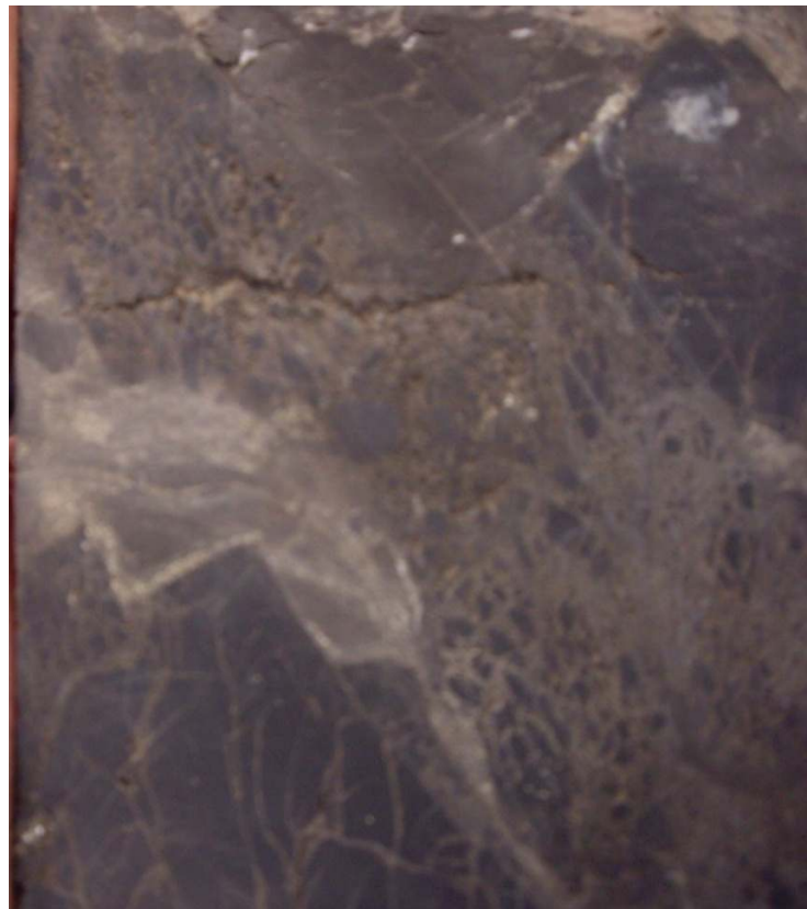
Image 100-574. Chert subunit showing the contact of chert and shale. Fracture pattern in shale matrix is evident due to pyrite cement. Width 4 inch. Drummond 1-N. Depth 3052-55 feet.
