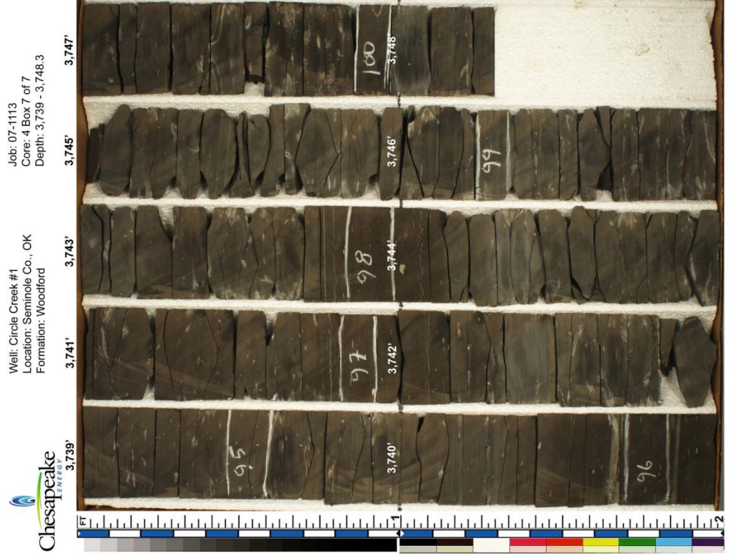
Appendix I. Circle Creek #1 core images: 3,729' – 3,748.3' (contact between Woodford Shale S2 and S3 indicated by yellow line)
