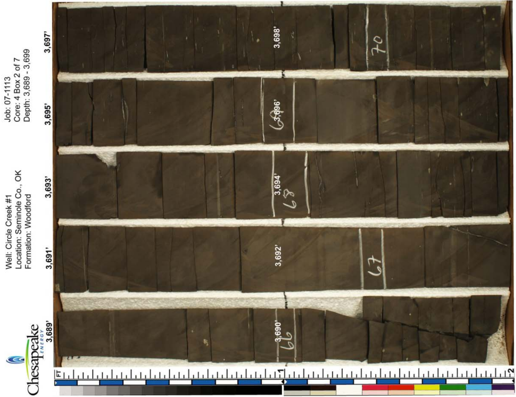
Appendix I. Circle Creek #1 core images: 3,689' – 3,709' (Woodford Shale S2), pyrite nodules indicated by yellow arrows
