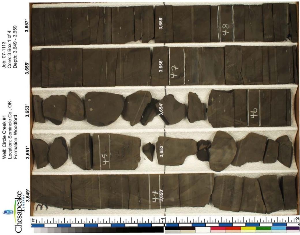
Appendix I. Circle Creek #1 core images: 3,649' – 3,669' (Woodford Shale S2), pyrite indicated by yellow arrow
