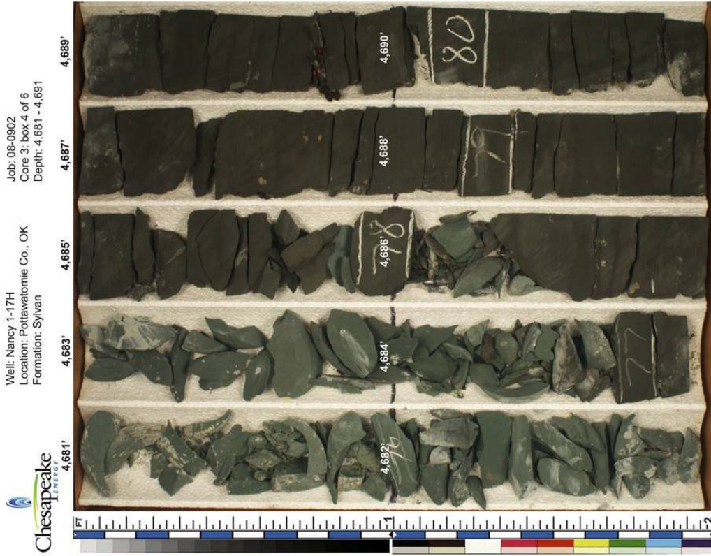
Appendix II. Nancy 1-17 H core images: 4,671' – 4,691' Contact between Hunton Group and underlying Sylvan Shale indicated by yellow line
