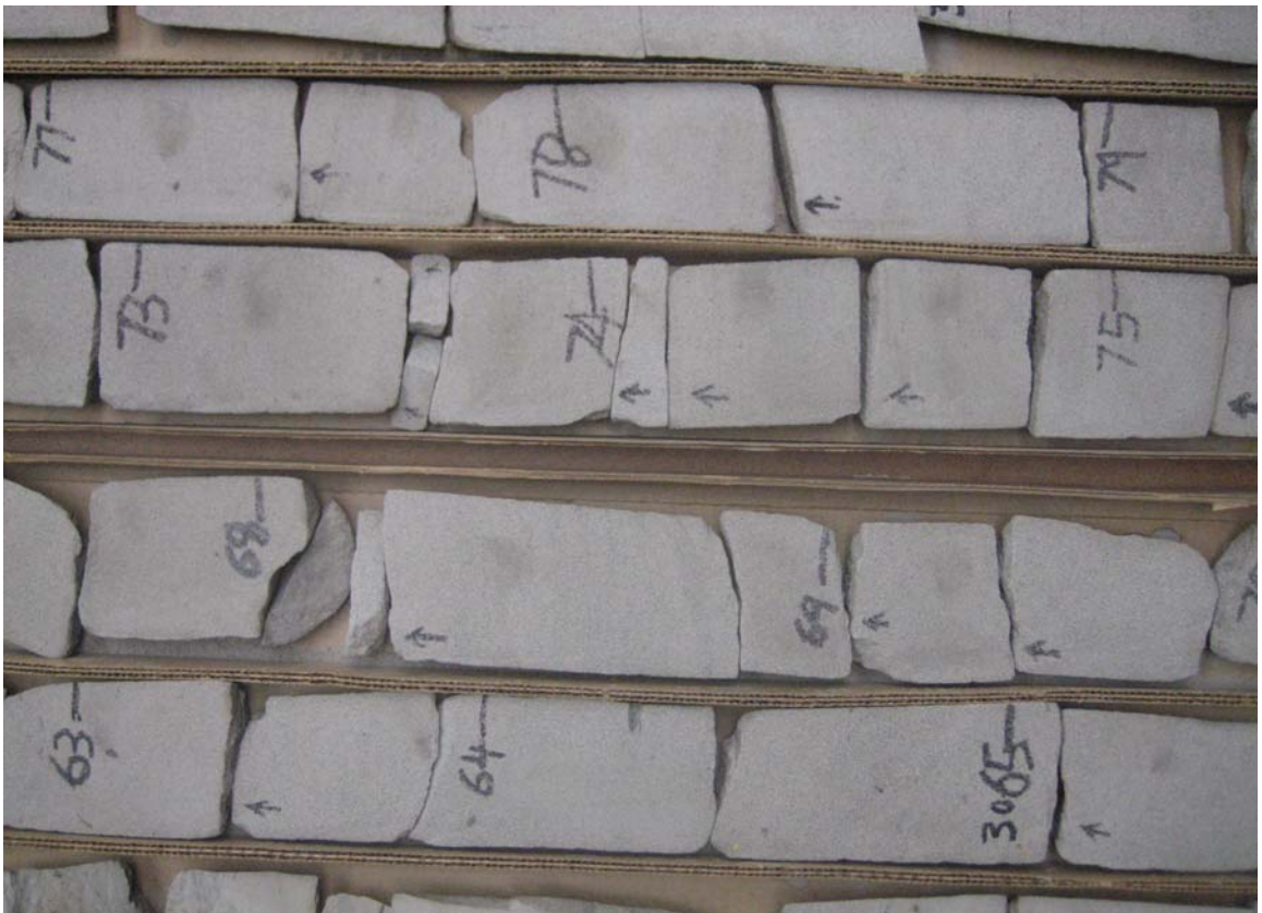
Figure 9: Example of featureless (massive) coarse grained sandstone that makes up the Lance Formation in the American Beryllium Oil Corp, Aspirin Unit 1 Depth 3063-69 feet.
