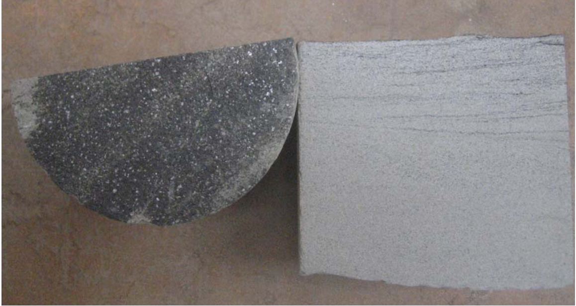
Figure 8: Coarse grained sandstone with dark mica and abundant carbonaceous material illustrating bedding structures. American Beryllium Oil Corp, Aspirin Unit 1, Depth 3045 feet.
