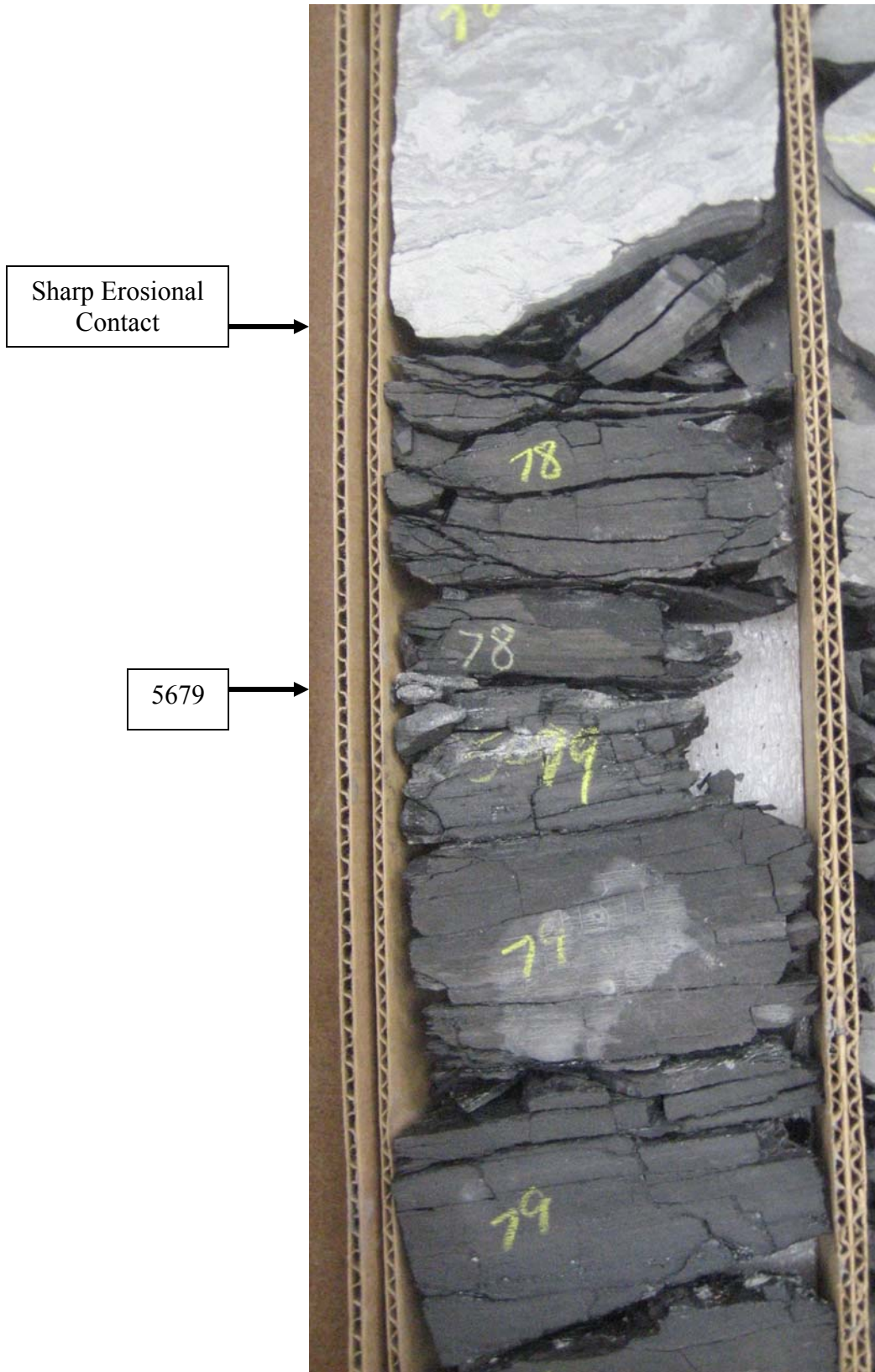
Figure 7: Sharp erosional contact between sandstone (light color) and underlying coal. Depth 5678 -5679 feet. Devon, BSU 11-13-19-63
