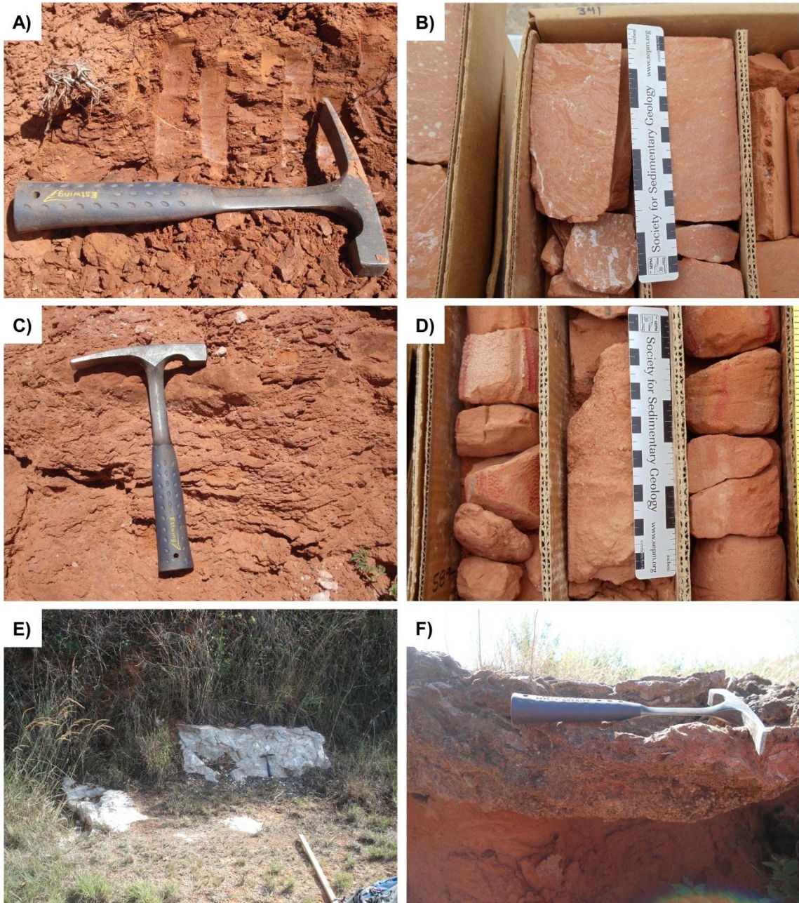
Figure 11. Extradune facies assemblage. A) Argillaceous sabkha facies, MS-14, B) arenaceous sabkha facies, in core MC-01, showing convolute bedding, C) arenaceous sabkha facies in outcrop, MS-22, showing ripple laminations, D) fluvial facies, MC-01, showing normal graded bedding. E) block of gypsum facies of Weatherford Bed, MS-17 and D) carbonate facies of the Weatherford Bed, MS-02.
