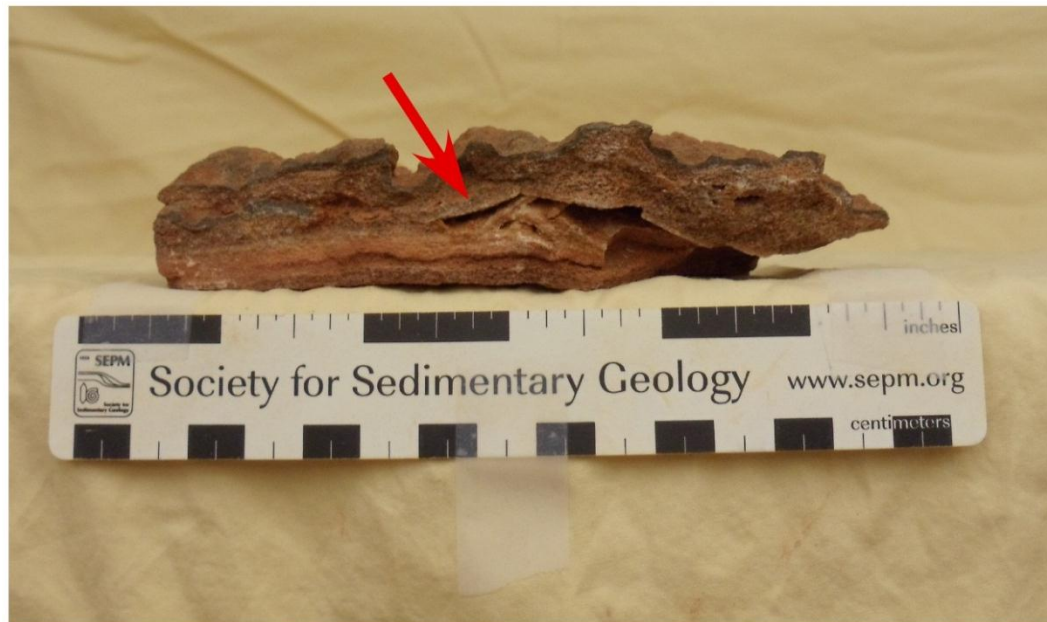
Figure 13. Carbonate facies of the Weatherford Bed. Hand sample taken at MS-02. Note laminated bedding and large sheet cracks (arrow).
