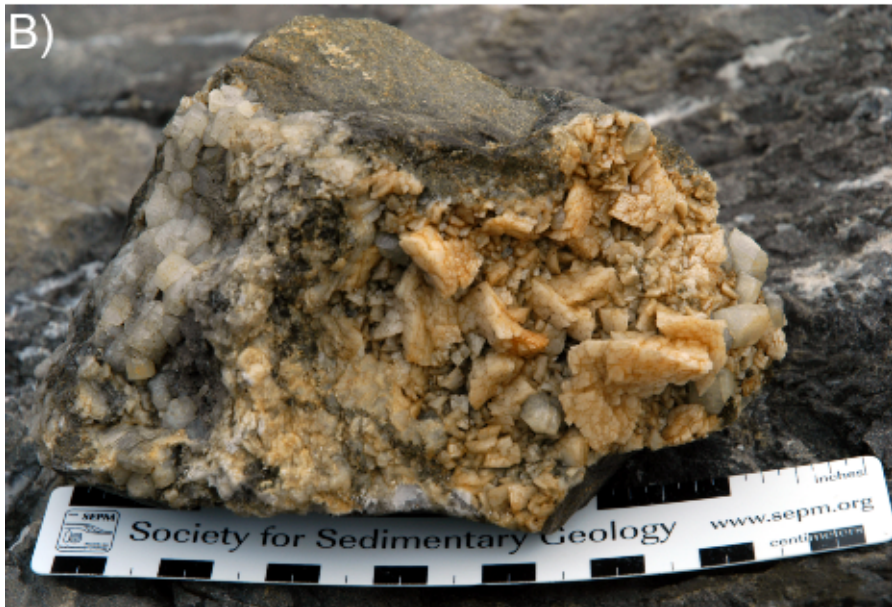
Figure 9. A) Hand sample showing two types of dolomite cements at Abbeytown: large (cm-scale), white-pink saddle dolomite (left) and small (< 1 cm), grey dolomite rhombs (right) [AM-11]. B) Large, white-brown saddle dolomite (right) with white calcite cements (left) from Abbeytown Mine [AM-10].
