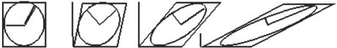
Figure 9: This diagram shows that simple shear involves rotation about a point.
