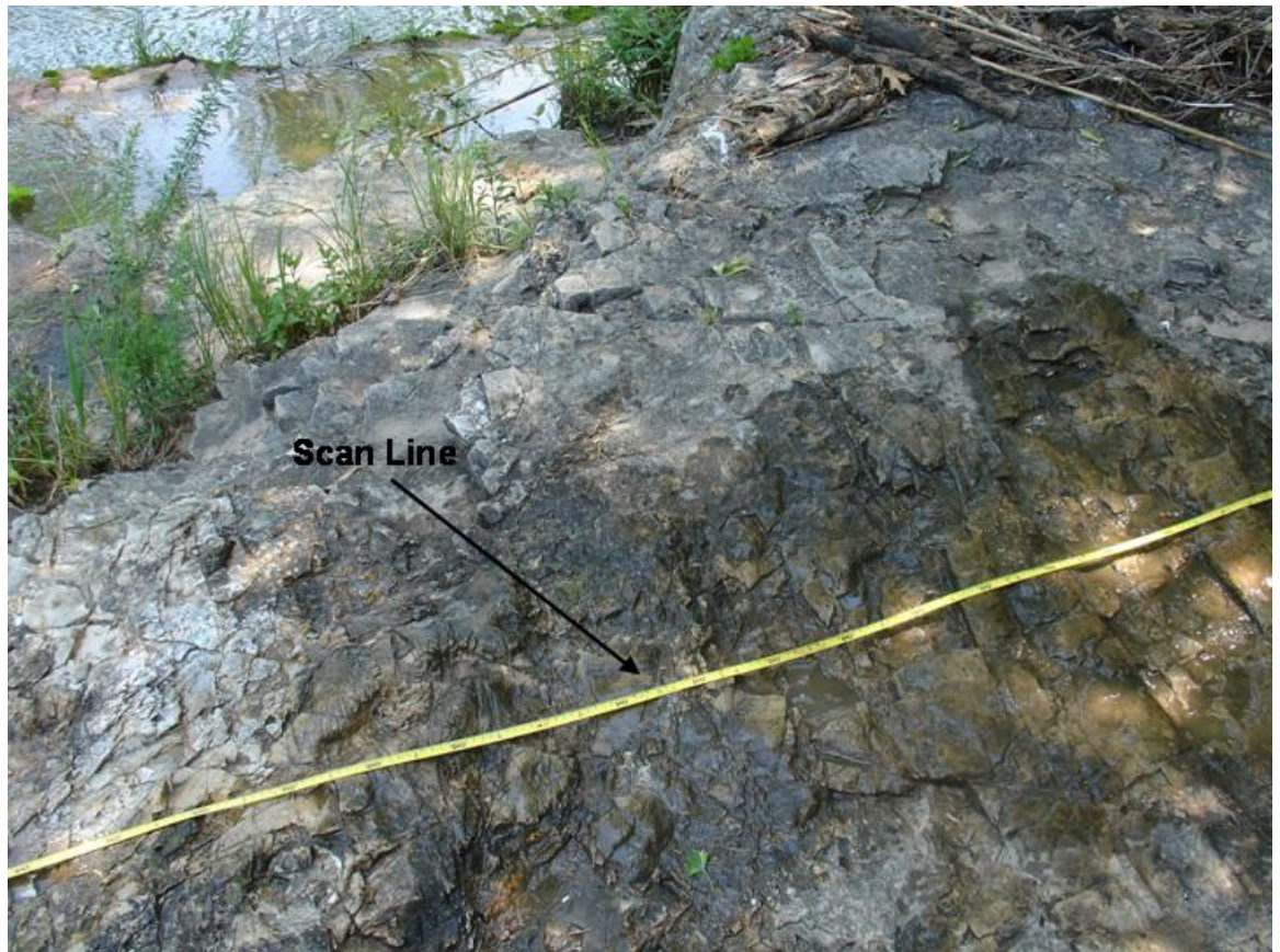
Figure 3-4. A scan line taken across fractures was used to gather data. One dominant trend is seen perpendicular to the scan line. A second fracture set can be seen parallel to the tape and has grass growing in one of the fractures in the set.
