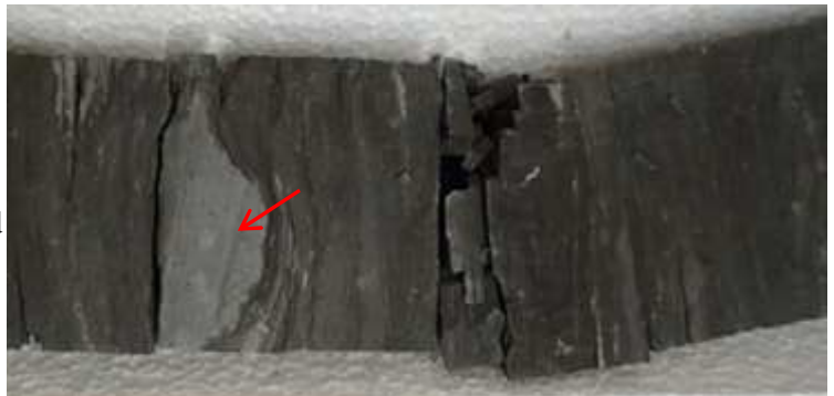
C6-002: Soft sediment deformation, Pillow of calcareous mud injected into non calcareous mudstone
