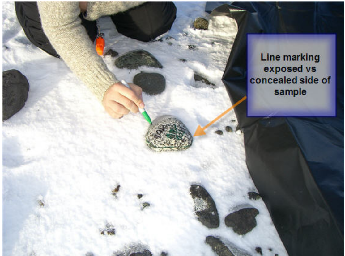
Figure 5. Illustration of labeling the top side of a sampled cobbles.
