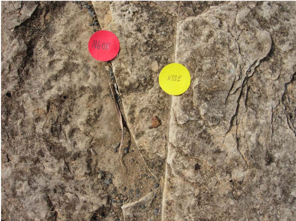
Figure 6: An example of a J-Junction, where a younger joint curves into the older joint acting as a free surface. Picture from the Bend River locality.
