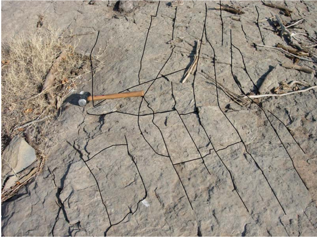
Figure 43: An example of how fracture orientations can be affected by a topographically low feature, which causes a change in the local stress field.
