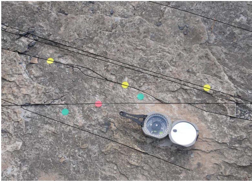
Figure 38: An example of fractures curving in the presence of a free surface. Displacements along the same fracture were never the same. Colored dots indicate sets of related fractures.
