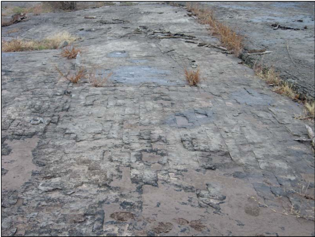
Figure 41: Picture illustrating fractures in Unit II with only one orientation.
