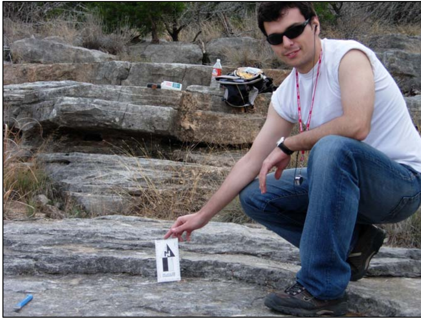
Figure 57: Thinner beds within the Honeycut contained significantly higher fracture intensities
