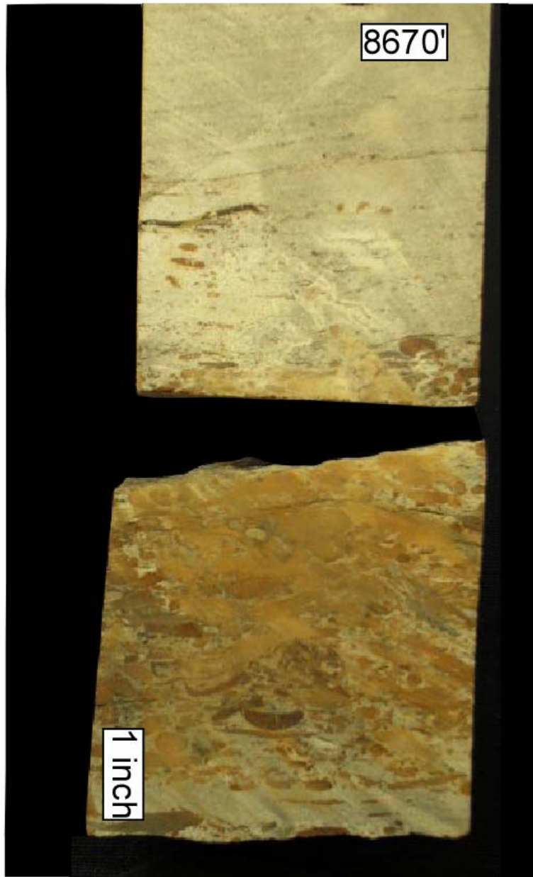
Figure 14. Basal rip-up clast conglomerate that grades upward into fine-grained, horizontally bedded sandstone. Mud rip-up clasts (channel lag) are common in high energy environments. Texaco, Payne No. 17-1.
