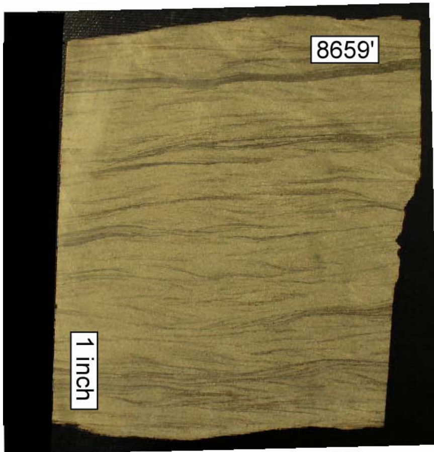
Figure 12. Very fine-grained sandstone with thin clay laminae. Sedimentary structures include ripple laminae and trough cross-bedding. Texaco, Payne No. 17-1.
