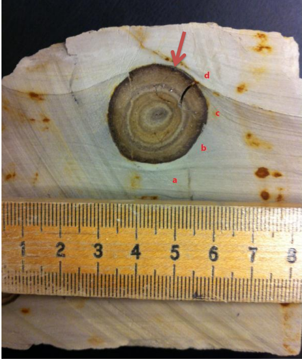
Figure 14: In situ phosphate nodules in host shale. Laminae instantly extend beneath the nodule (a), then abut the nodule (b), lap against the nodule (c) and upper extends across the nodule (d) (arrow points to fore mentioned nodule).
