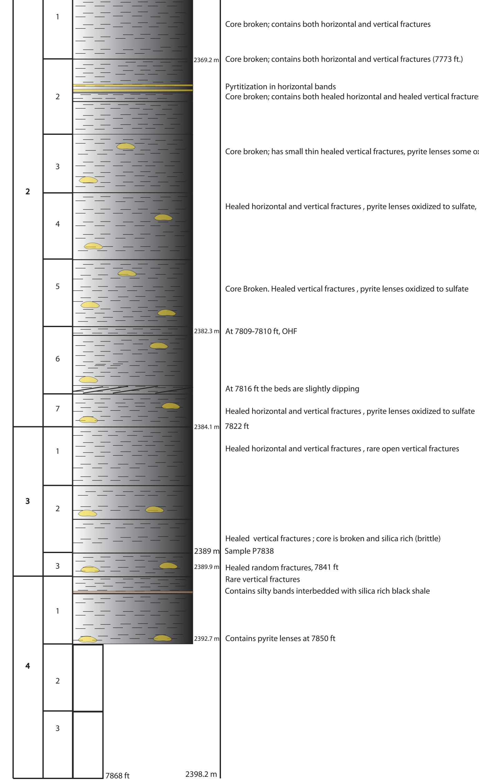
Core broken; contains both healed horizontal and healed vertical fractures
